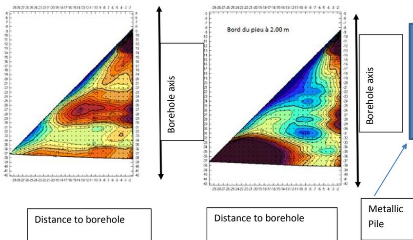
Figure 11: Case of a magnetic pile vs Natural ground (left)
