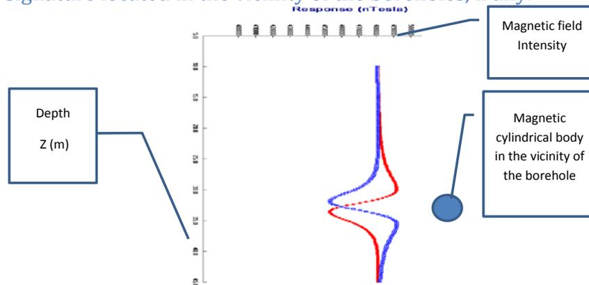
Figure 10: Case of a magnetic cylindrical body
