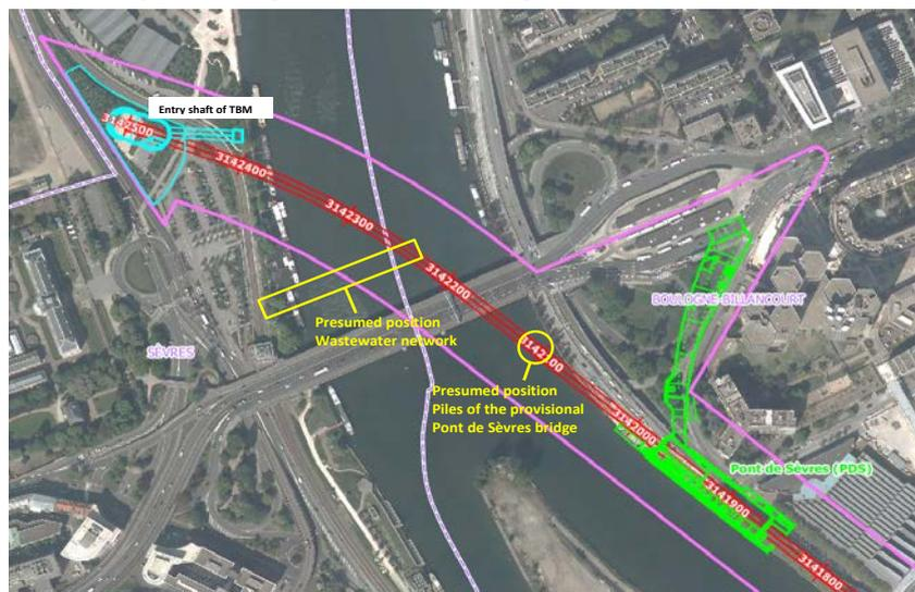
Figure 3: Localization of the remains of the two structures situated under the Seine bed
