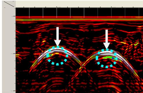
Figure 12: Example of two buried structures detected with GPR
