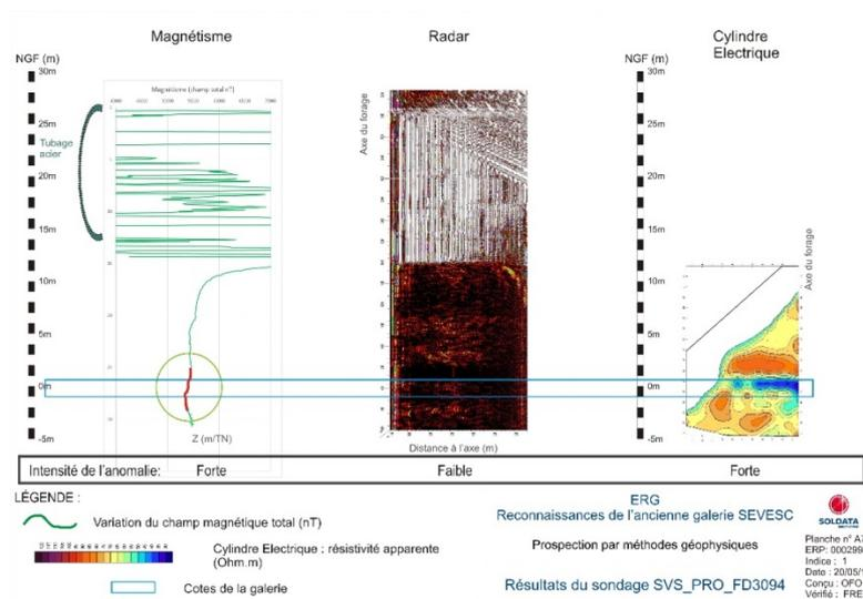
Figure 13: Case of a magnetic pile vs Natural ground (left)
