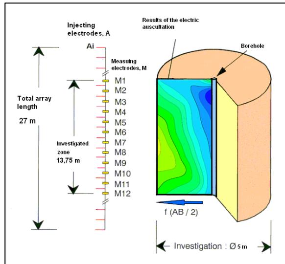
Figure 7: Electric Cylinder™ principle
