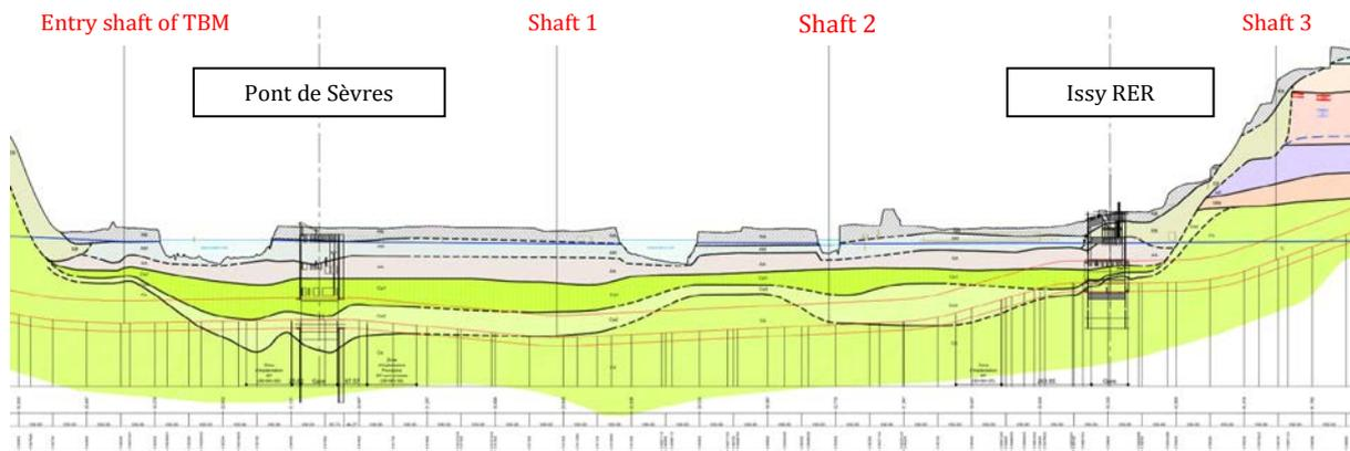
Figure 2: Geological profile of the « Seine Valley » part of the line 15-South
